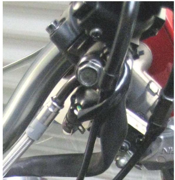
**Clutch cable (3):** Use the new clutch cable and route it as the original.
